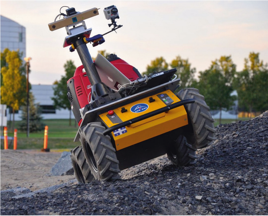
Fig. 4.13. Clearpath Husky robot with differential drive steering (photo by Tim Barfoot)
