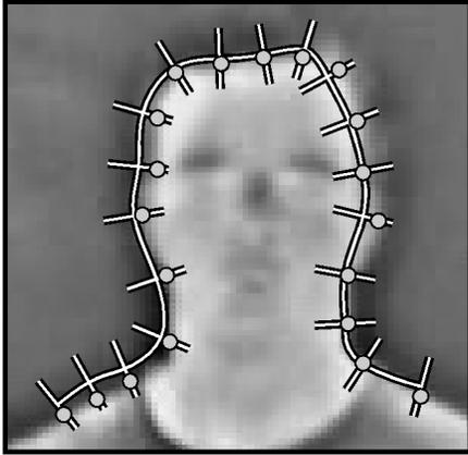
Fig. 3. Snake. State of a sample snake head tracker (infrared image). Circles on curve normals indicate locations of strongest Sobel edges.
