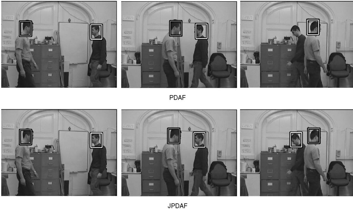
Fig. 11. JPDAF vs. PDAF: Tracking crossing homogeneous regions. Frames 0, 12, and 24 are shown.
