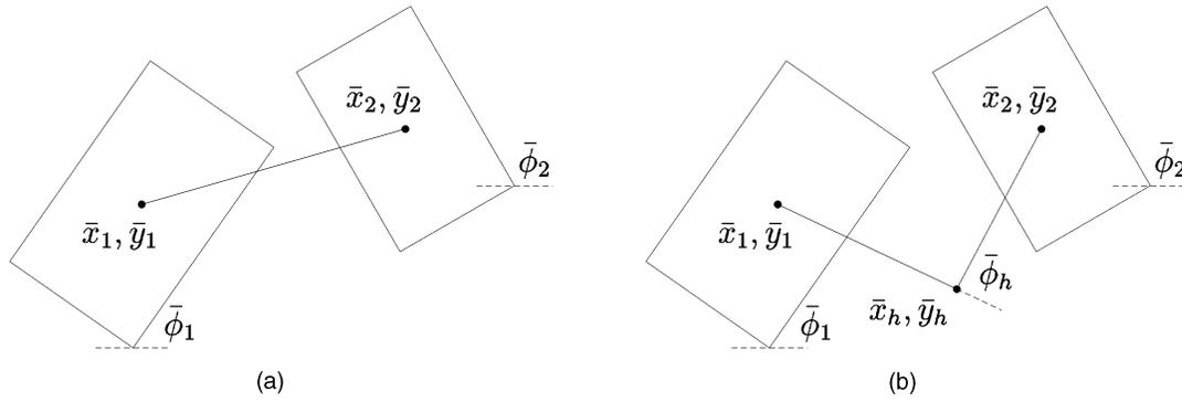
Fig. 6. Constraint types. (a) Initial configuration of a rigid link. (b) Initial configuration of a hinge.
