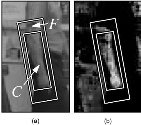
Fig. 1. Homogeneous region. (a) The geometry of a region for an arm tracker with the positive center  $C$  and inhibitory frame  $F$  labeled. (b) Pixel similarity  $\gamma$  of the image to the modeled arm skin color, with  $R$ 's geometry overlaid. (Input image courtesy of J. MacCormick).
