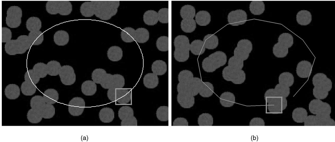
Fig. 7. PDAF: Tracking a homogeneous region with uniform noise (CG). (a) Frame 0 with initial position and ground truth of path overlaid. (b) Frame 300 with history of estimates at 25 frame intervals.
