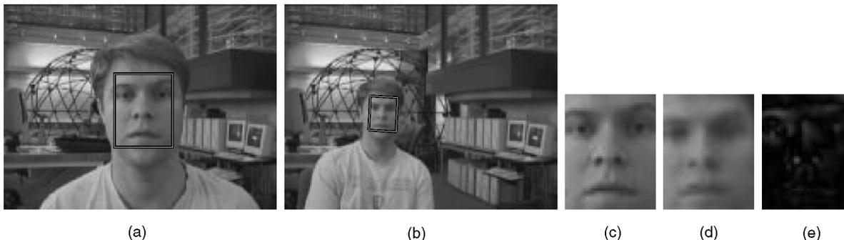
Fig. 2. Textured region. (a) Selecting the reference image for a face tracker. (b) One possible state. (c) Reference image  $\mathbf{I}_R$  from (a). (d) Normalized comparison image  $\mathbf{I}_C$  for the state in (b). (e) Difference image  $|\mathbf{I}_R - \mathbf{I}_C|$ .
