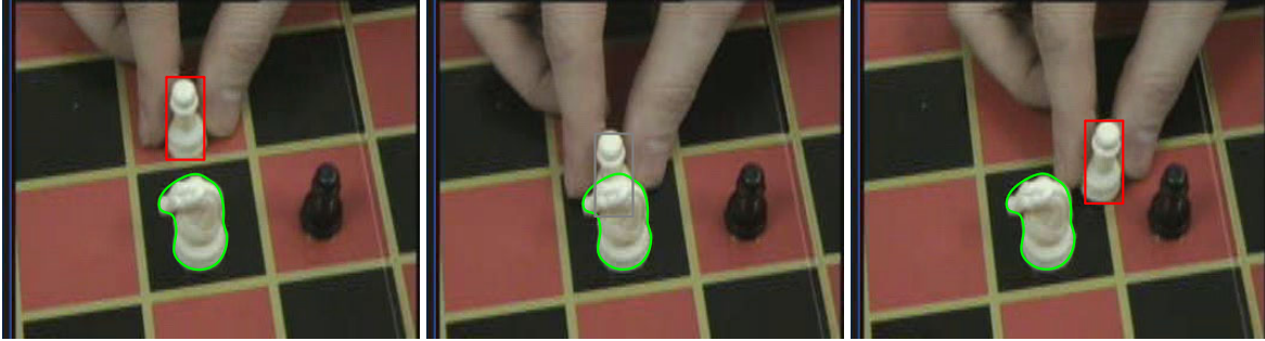
Figure 3. JLF (frames 0, 40, and 80). Deducing the occlusion relationship between a textured region and snake.
