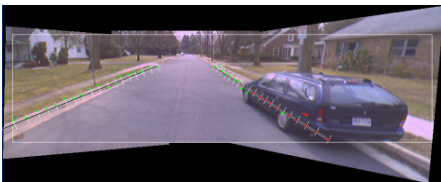
Fig. 5. Polycamera mosaic obtained by manual correspondence for road following.
