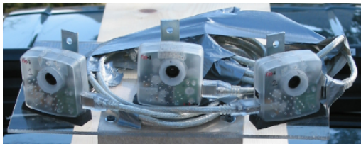
Fig. 2. Polycamera consisting of 3 cameras
