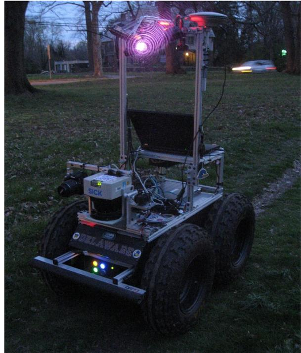
Fig. 1. Robot at night with twin Kinects active
